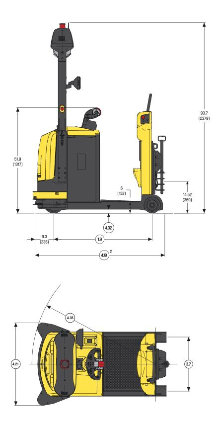
Circled dimensions correspond to the line numbers on the tabulated chart inside the technical guide. Dimensions are in inches (millimeters).
