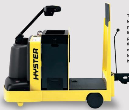
This Hyster T5-7ZAC Tow Tractor series features a resilient high-impact thermoplastic cowl cover that won't crack or break. It provides excellent protection against potential damage to internal components like the motor and electronic controls. The top cover is fastened with "snap-fit" spring clips for quick, easy removal. The bottom cover is held in place by 3 screws.
