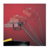
3-position tilt steer column helps give you comfort and stability. T5-7ZAC Tow Tractor is shown with the 17-inch wide control handle equipped with the optional "Side Glide" feature.
