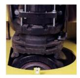
Sealed and bathed in oil, the Master Drive Unit (MDU) bearings provide quiet, smooth, low-effort control.
