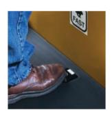
Mounted in the floor plate, the high speed or "rabbit" speed switch gives the T5-7ZAC Tow Tractor excellent travel speeds, helping to increase productivity.
