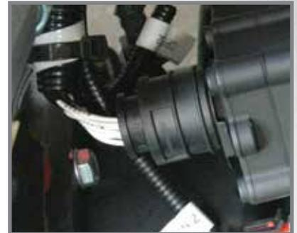
*Standard profile Deutsch pin connectors, IP64 compliant*
