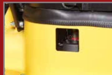
*Hydraulic sight gauge for fluid level checks*
