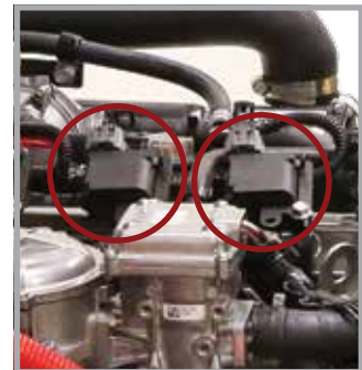
Coil over plug ignition design
