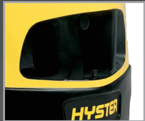
Counterweight tunnel design improves airflow
